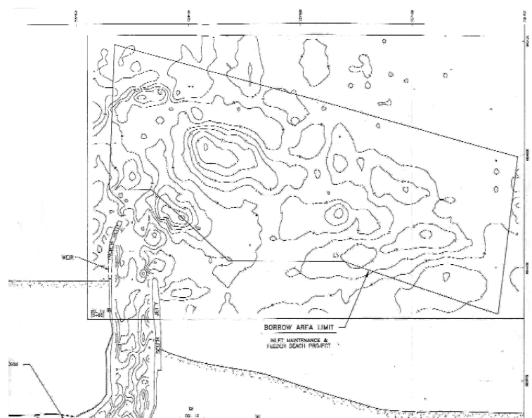
Borrow Area Hydrographic Survey
