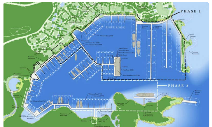
CSI designed the marina facility to accommodate 118 slips with over 11,000 linear feet of mooring space.
